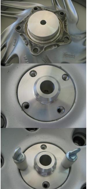
Slide the adapter in from the drive side of the rear wheel.
