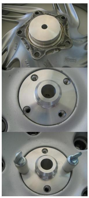
Slide the adapter in from the drive side of the rear wheel.
